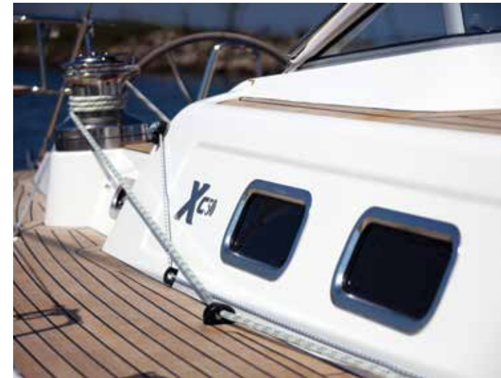
All the sheets run smoothly to the cockpit standard self-tailing stainless steel winches.
