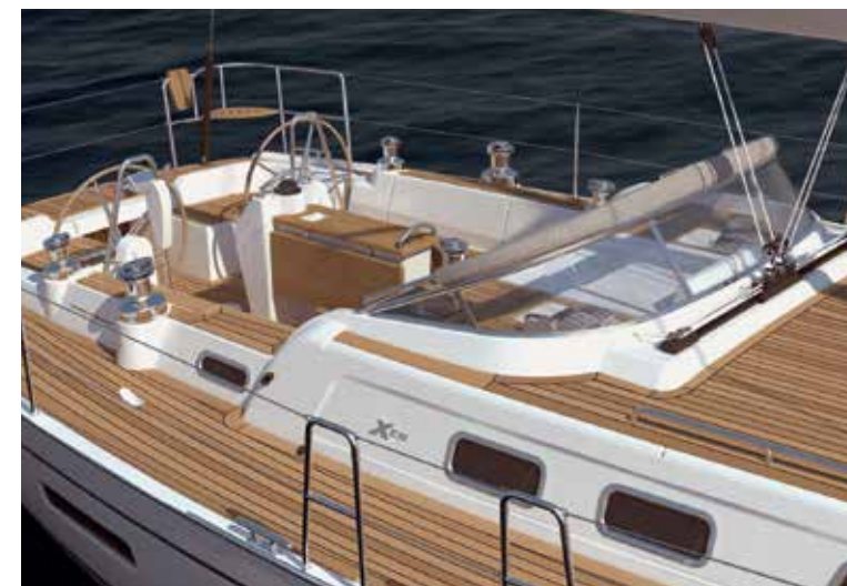
Xc 50 comes optional with an aluminium framed windshield with toughened glass.
