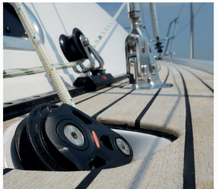
Optional vacuum applied teak side deck. German mainsheet passes below deck on both sides and is led back to the aftmost cockpit winches.
