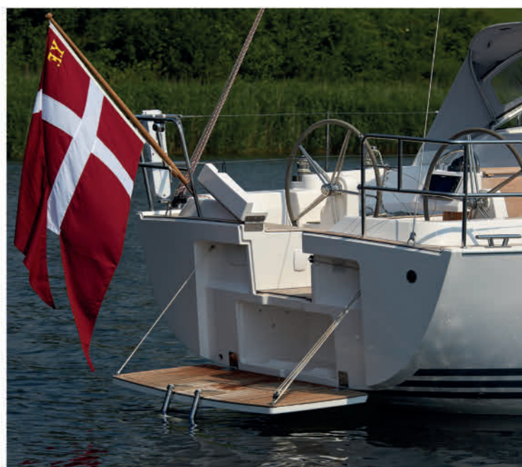
The large bathing platform is operated by a purchase block system. Below deck storage for a liferaft is accessed from the bathing platform.
