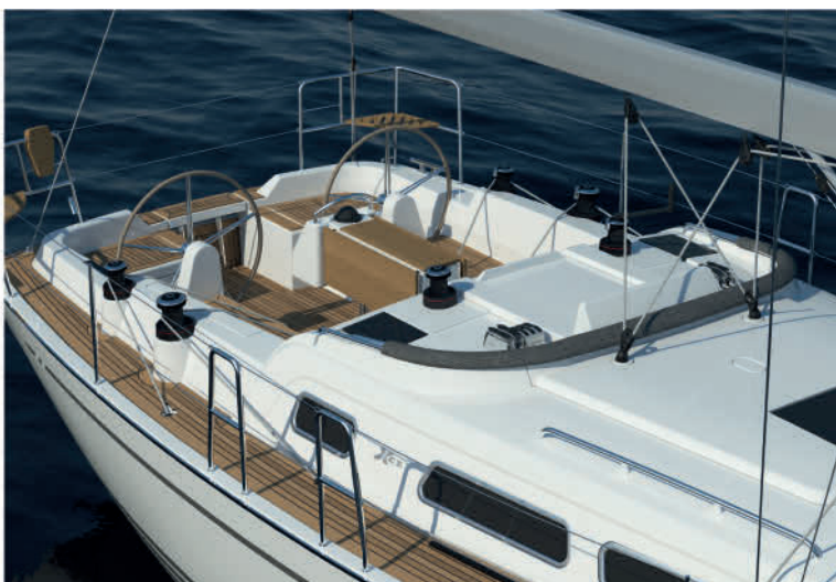
The optional spray hood rests in a "sock" when folded. The aft pushpit teak seats are optional.
