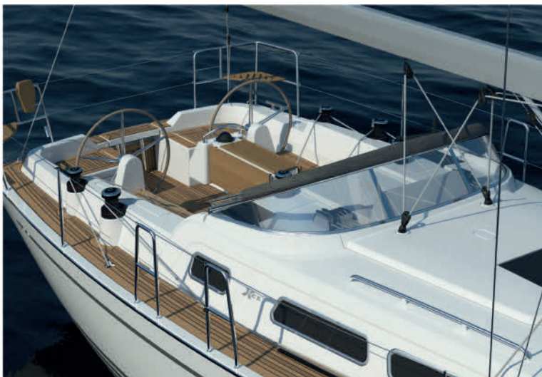
Xc 35 comes optional with an aluminium framed windshield with toughened glass including a stainless steel framed spray hood.
