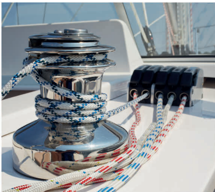
The Xc 35 comes standard with 6 self-tailing Harken winches. Optional stainless steel Andersen winches are available as an upgrade.
