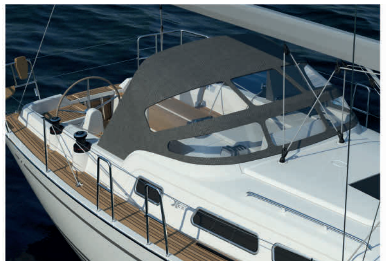
The optional spray hood is supported by three stainless steel frames. For canvas colour options, see page 17.
