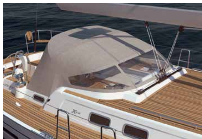
The spray hood is supported by stainless steel frames. For canvas colour options, see page 17.
