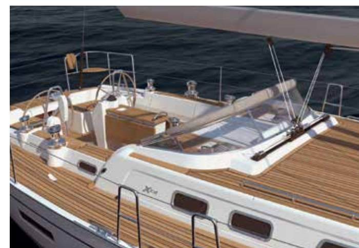
Xc 38 comes with an aluminium framed windshield made from toughened glass including a stainless steel framed sprayhood.
