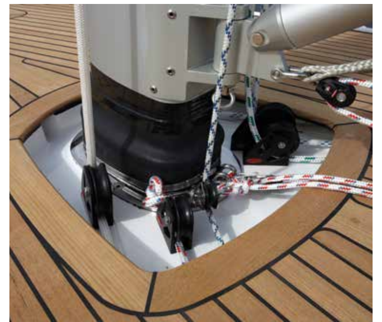
Optional vacuum applied teak on the coachroof. Split mainsheet passes below deck on both sides and is led back to the aftmost cockpit winches.
