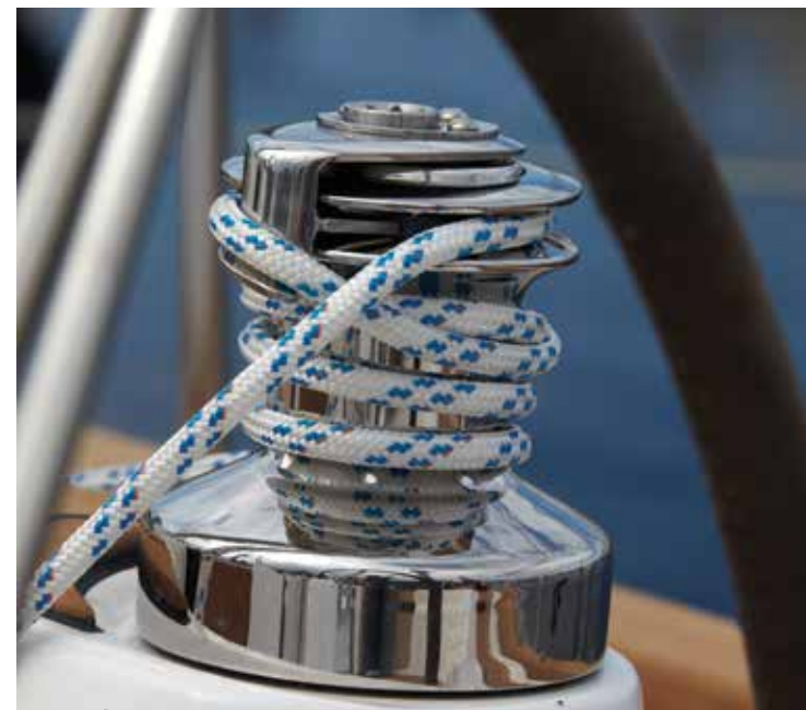
The Xc 38 comes standard with 6 self-tailing Harken winches. Optional stainless steel Andersen winches are available as an upgrade.
