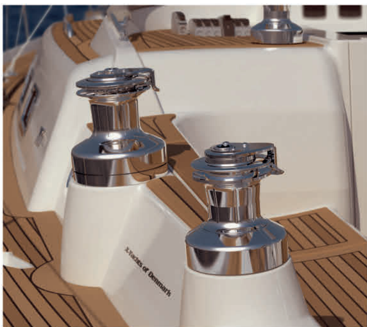
Stainless steel self-tailing Andersen Winches, which can be upgraded to be electrical powered are part of Xc 42's comprehensive standard quality.
