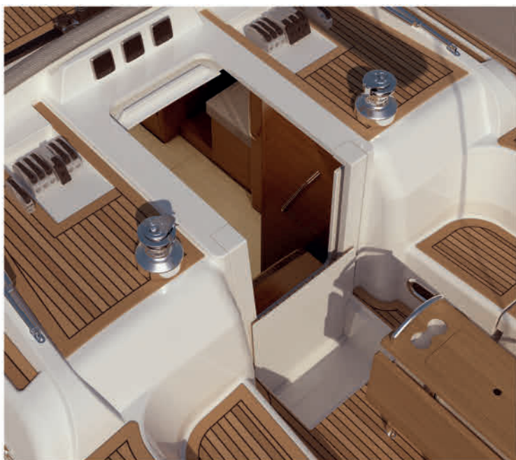
All halyards pass below the deck surface and are stored in the cockpit floor self draining "bin". Self-draining, acrylic dropboard is supported by gas struts for easy adjustment.
