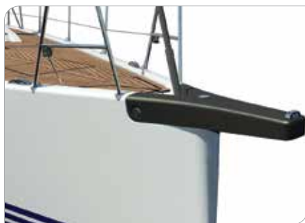
Optional carbon bowsprit without anchor
