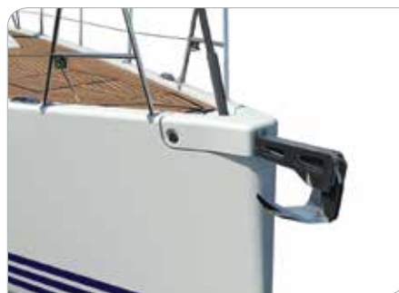
Standard GRP cowl with integrated anchor fitting
