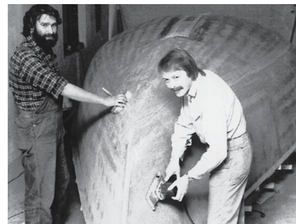
Niels Jeppesen and Birger Hansen building the hull plug for the first ever X-Yachts model, the One Design X-79. Almost 500 X-79s were built between its launch in 1979 and the mid-1990s
