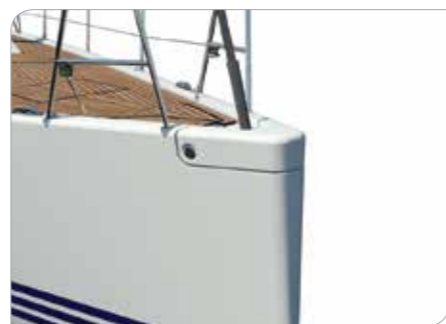
Optional GRP cowl for rating efficiency
