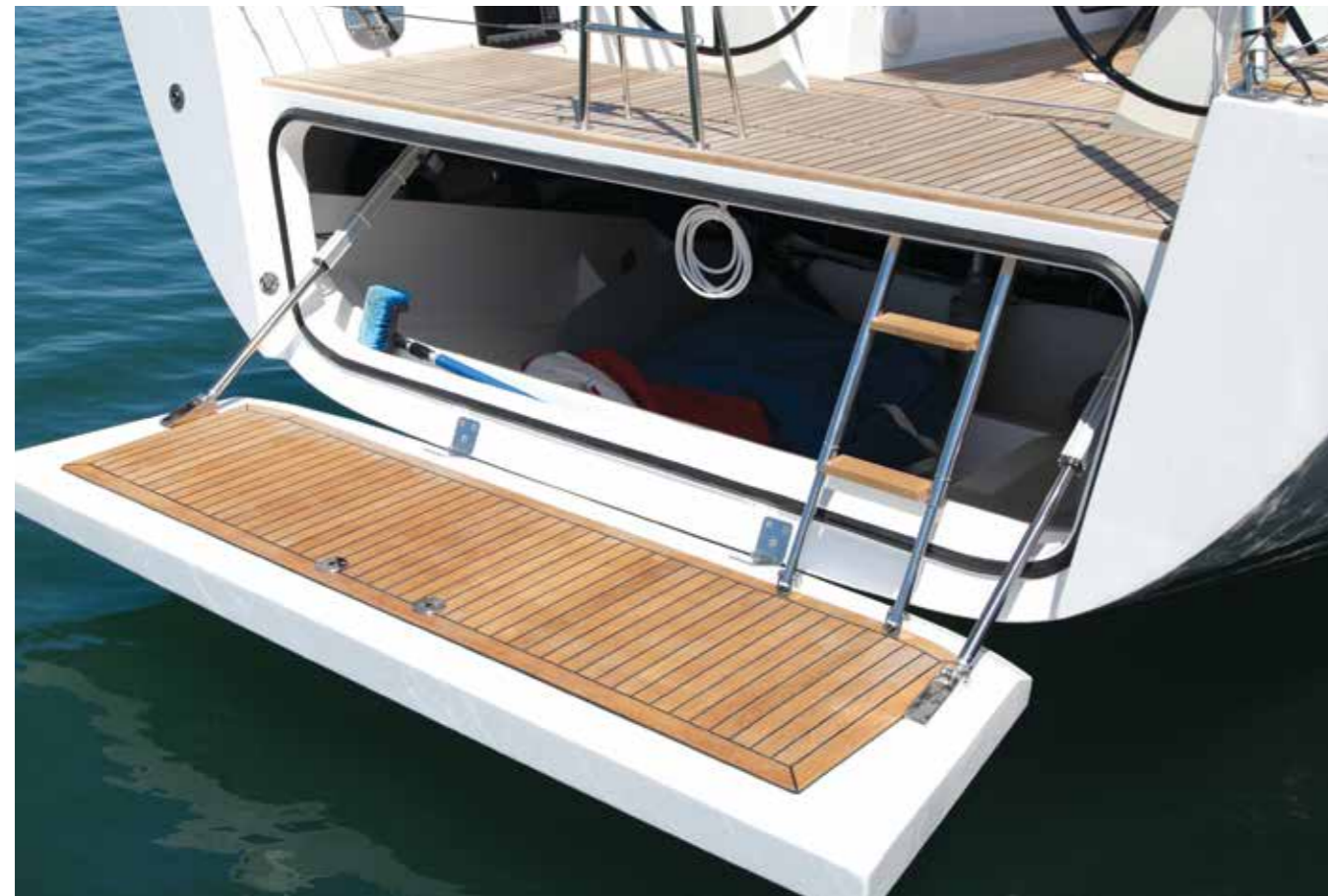
Electrically operated folding transom
