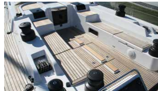
Dismountable cockpit floor foot chocks
