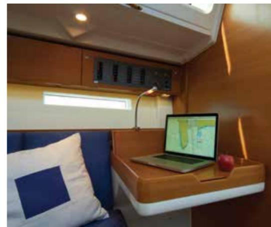
The Xp 38 features a sliding navigation station as standard, shown in forward (see above top) and aft (above) positions
