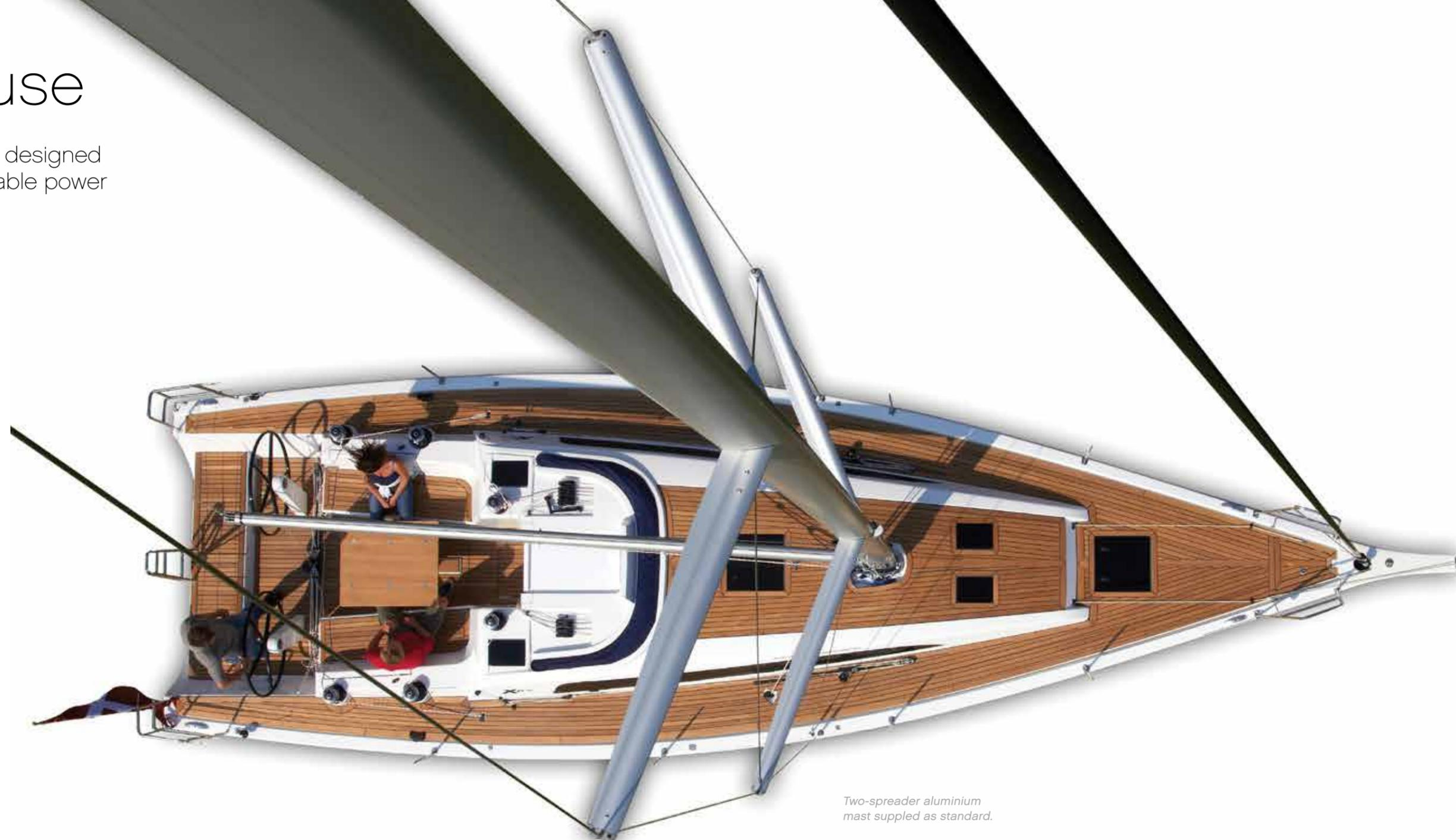
Two-spreader aluminium mast supplied as standard.
