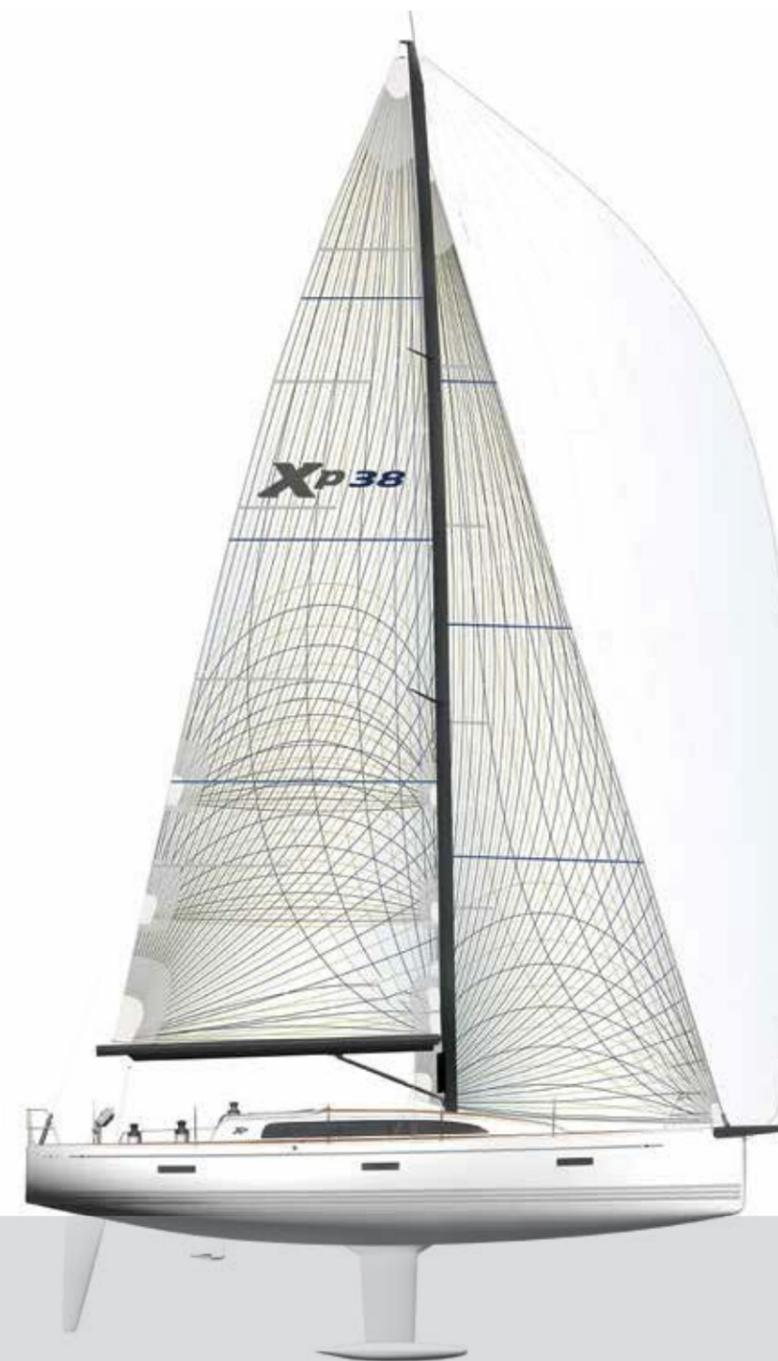
Xp 38 carbon rigs are developed utilising software which interfaces with leading sailmakers' design software to produce the optimum sail and rig combination (Source: Southern Spars)
