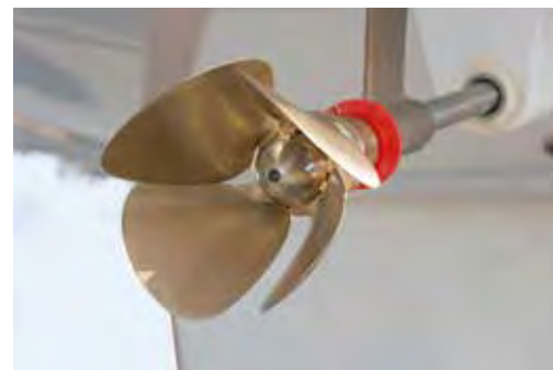
Flex-o-Fold 4-blade folding propeller / Hélice repliable 4 pales
