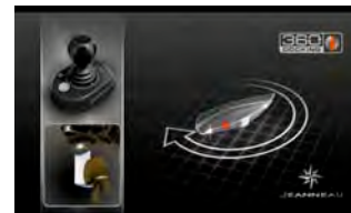
> Rotation: saildrive turns 90° to pivot boat around axis
